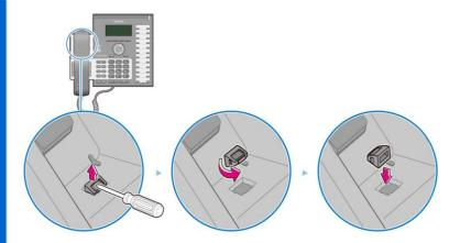
Attach to match wall mount bracket hole and screws, and pull down to make sure firmly fixed.
